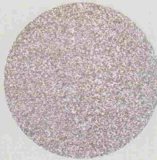
Primary Aluminium refined with AlTi5B1 (*) (Grain Size 100µ)
